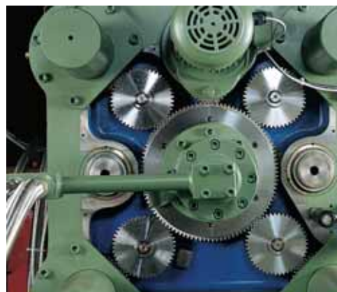
Motorised die height adjustment system.
