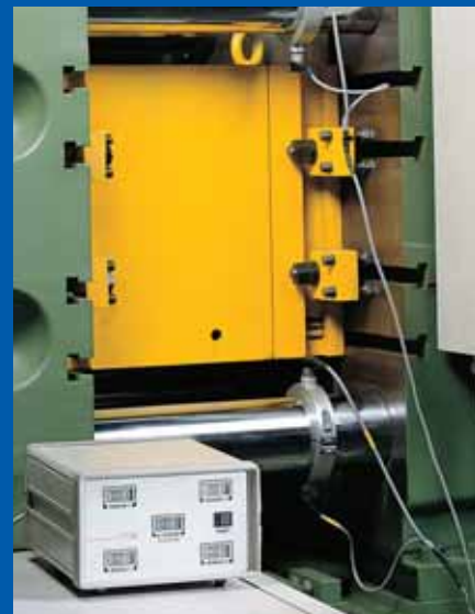
Die locking force test & Tie bar strain value analysis.
