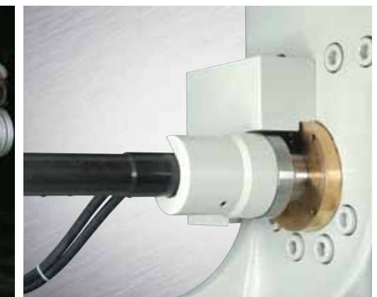
Shot stroke measuring by sensor rod.
