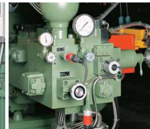
Shot speed control is read by precision scale gauge.
